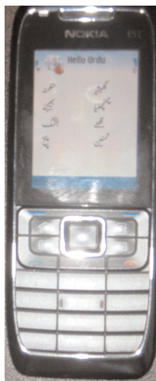
Figure 4: Pango Urdu (Open Type Font Nafees Nastalique) text rendering on a Nokia E51
