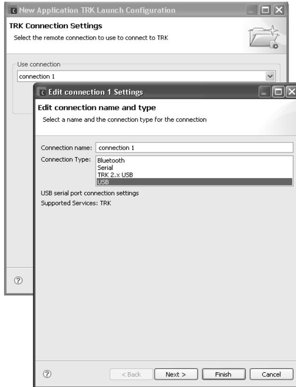
**Figure 4.25: Configuring Connection to the Device**
