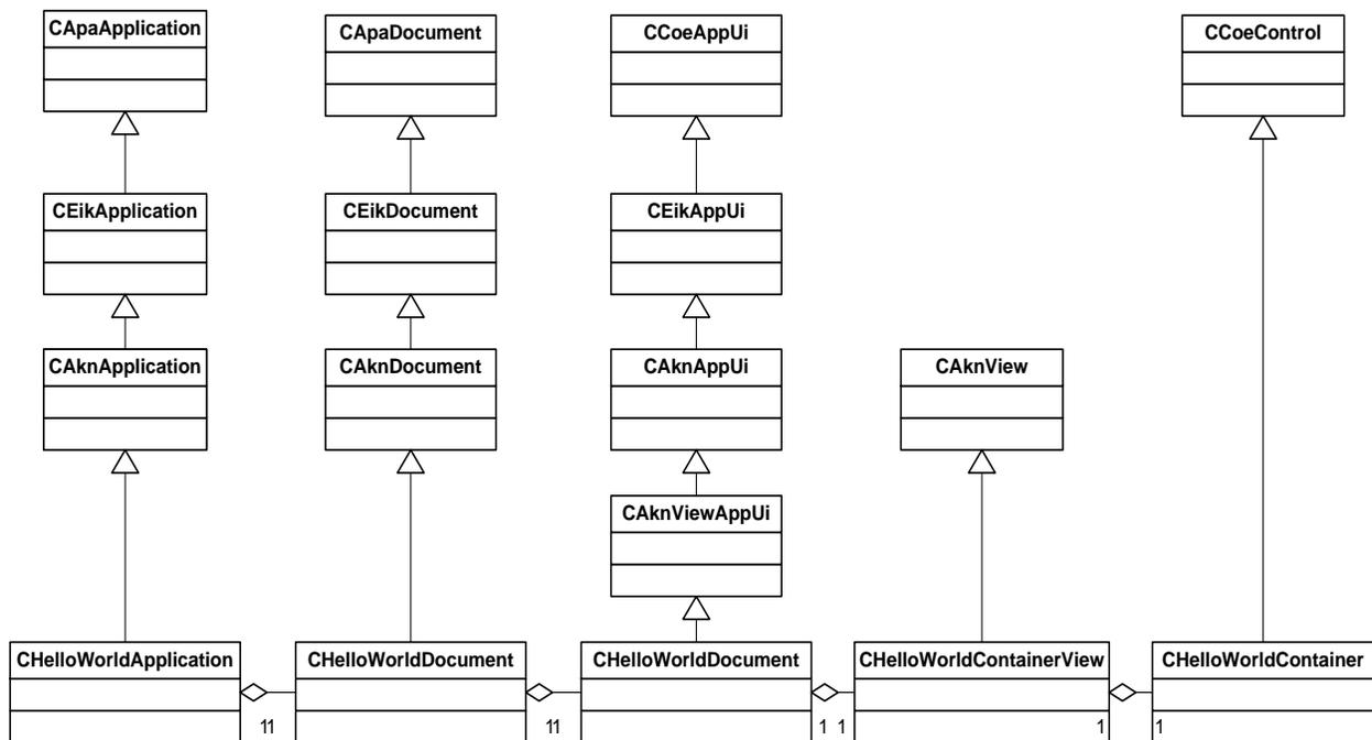
**Figure 6.1: HelloWorld View Switching Application Architecture**
