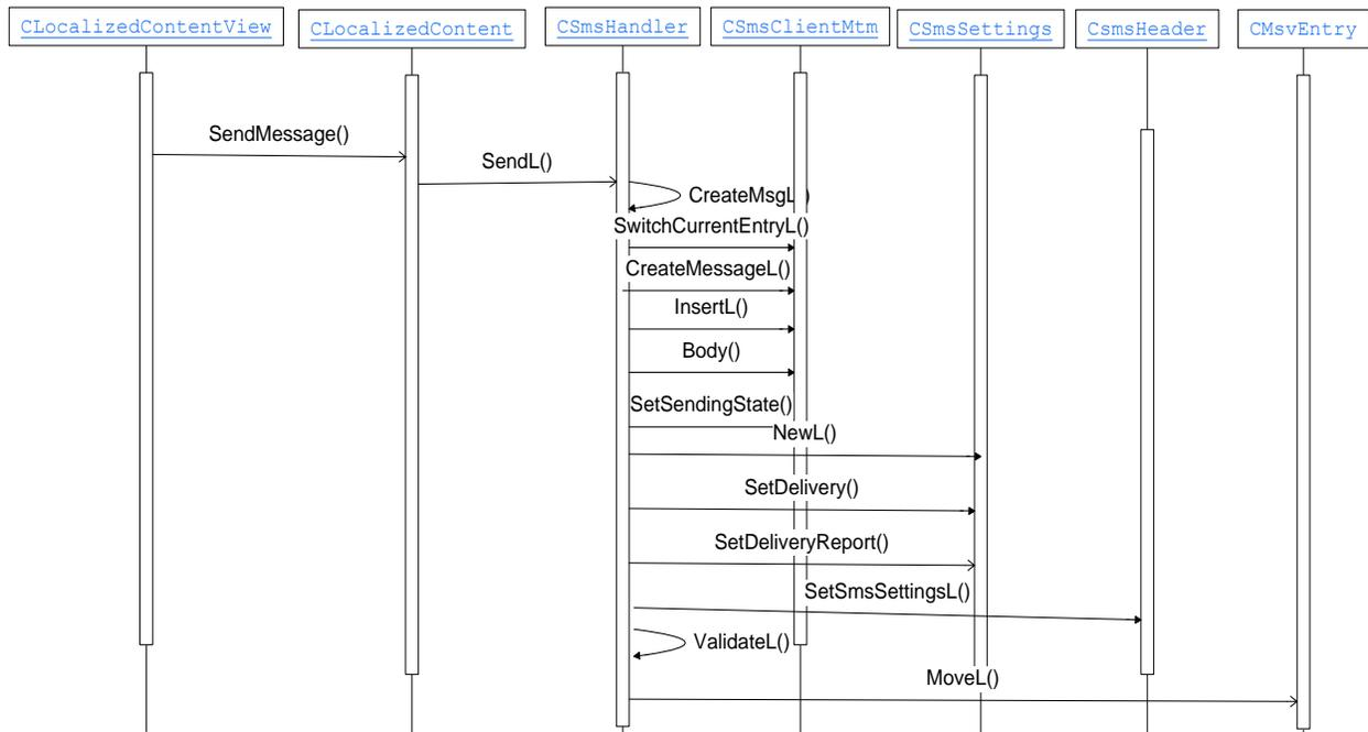
Figure 7.4: SMS send sequence diagram
