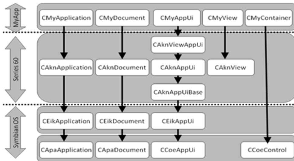
**Figure 5.4: View Switching Architecture**
