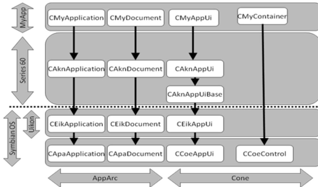
Figure 5.2: Traditional Symbian OS Control-Based Architecture
