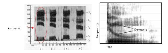
Figure 7: Spectrogram showing Formants
